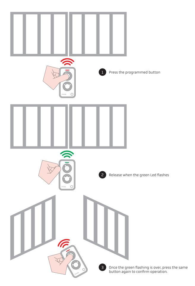
**Attention!** It is possible that at the end of the whole procedure it may be necessary to press the button on the original remote control several times until it works again.
